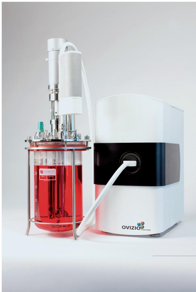
The previous version of the BioConnect used to be plugged directly onto the headplate of a benchtop, glass and steel bioreactor using a compression fitting. However, with the emergence of new cultivation methods, the BioConnect has evolved in order to accommodate not only benchtop bioreactors, but any type of cell cultivation vessel.
